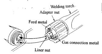
Surely insert the feed metal fitting and gas connection metal fitting of the welding torch and the wire feeder, check that the adapter nut is screwed in smoothly, and tighten. (If screwed in forcibly, the threads might be broken.)
