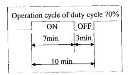
●If exceeding the rated duty cycle of welding power source and torch, temperature rise of welding power source and torch exceed the allowable temperature, and it can be a cause of burning.
