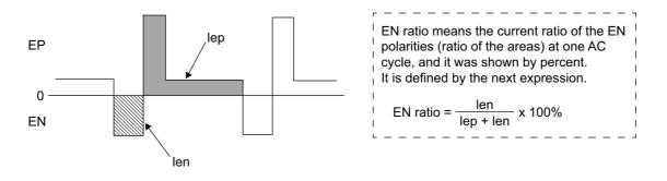
The EN ratio changes about 1% by adjustment amount '1' of the operation. A standard value of the EN ratio (value at center position '0') and the maximum value and the minimum value of the EN ratio are different depending on the welding process and each current setting.
