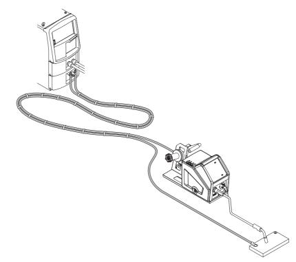
• When using the welding power source with surplus cables wound, wind them referring to the following good example.
