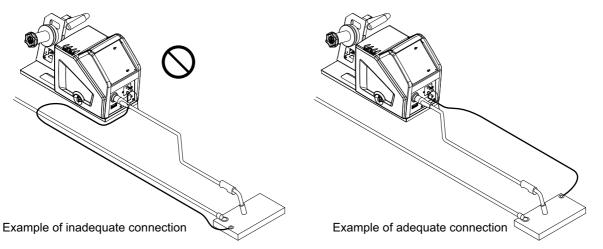
• Wire the voltage detection cable of the base metal side close to the one at the torch side (detection wire) to narrow the area surrounded by the two voltage detection cables.
