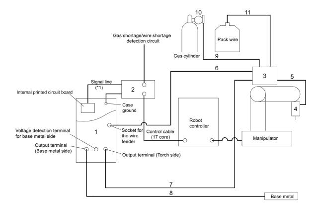
\*1: The welding power source is equipped with a built-in interface.
