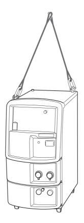
2. Lift the welding power source carefully paying attention to the balance by using lifting lug.
