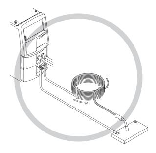
1. Divide surplus cables to A and B and wind them in the same manner, times of winding, and diameter.
