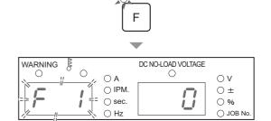
2. Turn the parameter adjustment knob, to display the function No. to set.
