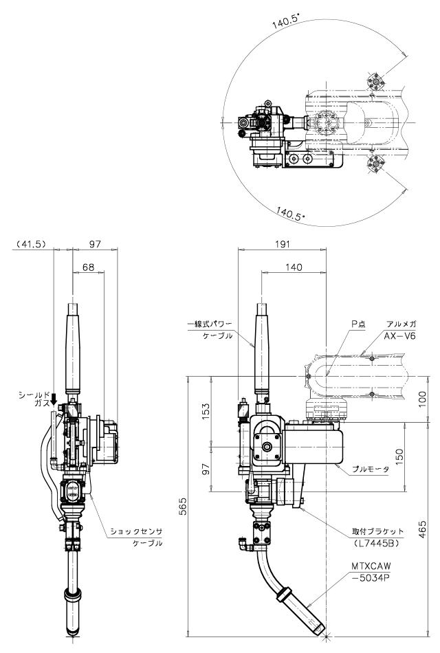
Fig. 1.3 Assembly drawing of pull feeder unit L-7591 + MTXC-3534P
