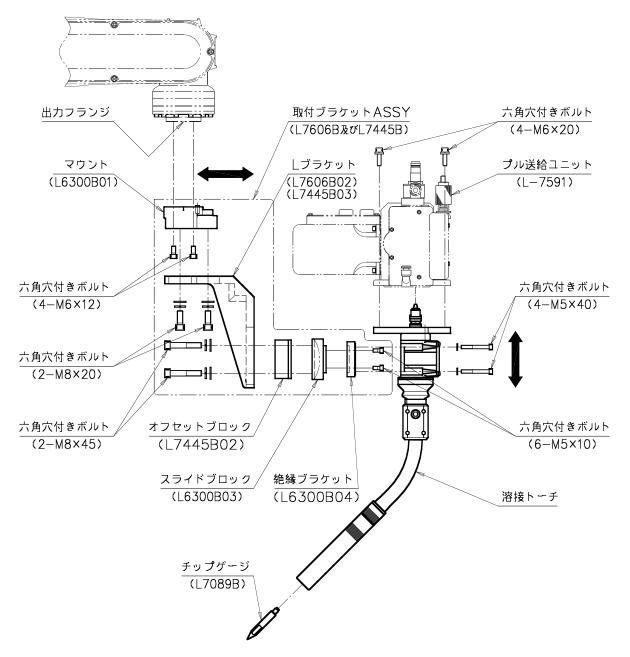
Fig. 3.1 Mounting torch (mounting bracket) and pull feeding unit
