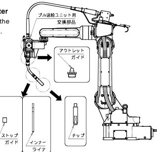
Fig. 6.1 Replacing parts in changing wire diameter
