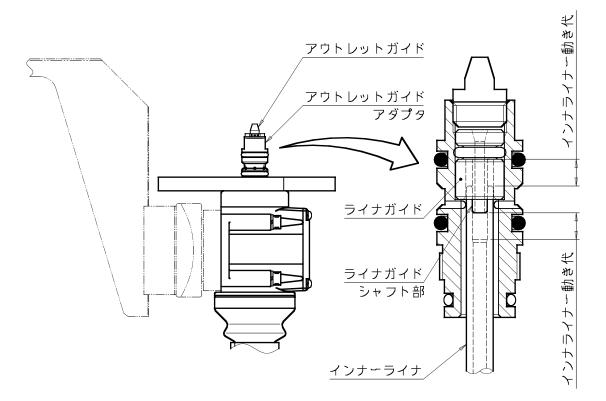
Fig. 6.6 Mounting of inner liner (in shock sensor)
