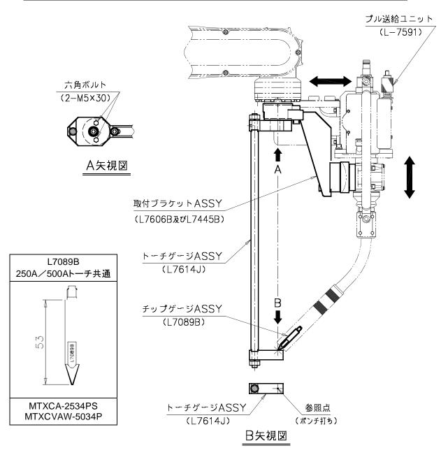
Fig. 3.2 Mounting torch gauge
