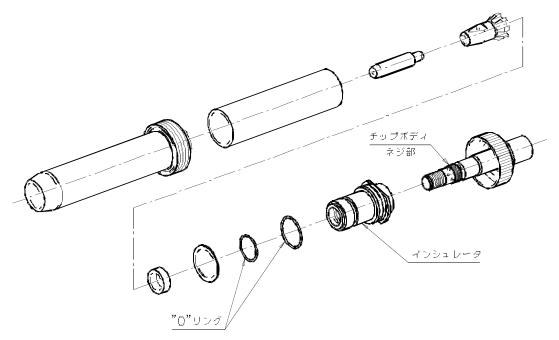
Fig. 6.8 Exchanging procedures of O-ring
