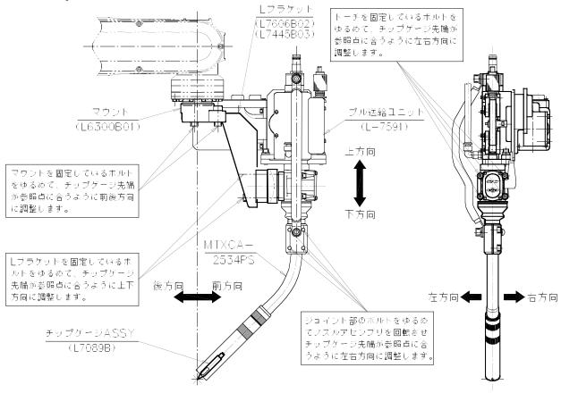
Fig. 3.3 Adjustment direction for torch
