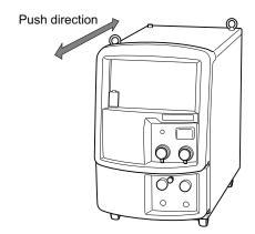
2. When using a tool such as carriers, secure the welding power source and carrier with a rope before transporting.
