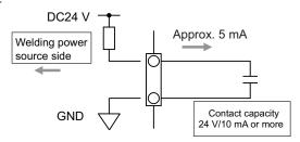
Output signal of the external connection terminal block
