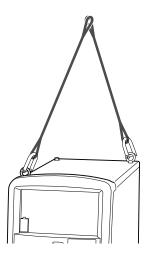
2. Lift the welding power source carefully paying attention to the balance by using lifting lug.
