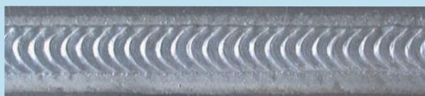
16 gauge (1.6 mm) A5052 Aluminum Plate Butt Welded With 3/64" (1.2 mm) A5356 Aluminum Wire
