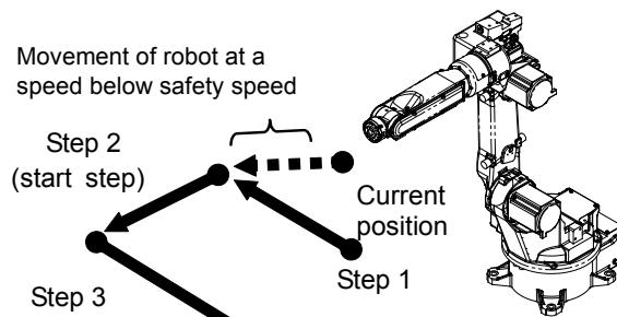
Fig. 5.1.1 Robot movements at safety speed
