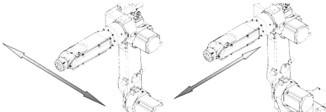
Fig. 1.4.3 Moving the robot tip in a straight line (robot coordinate operation)
