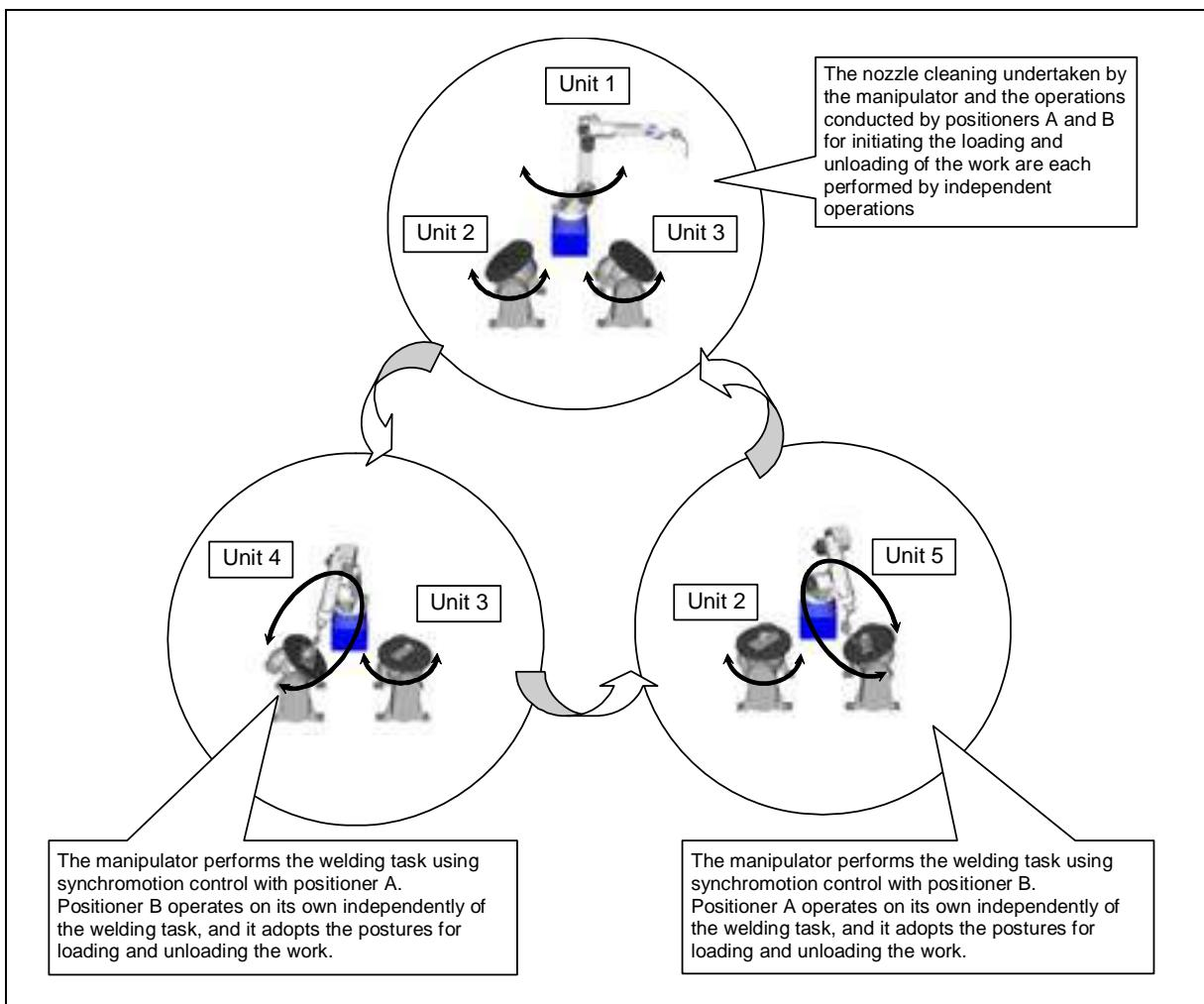
Fig. 7.1.1 Example of multi-task configuration
