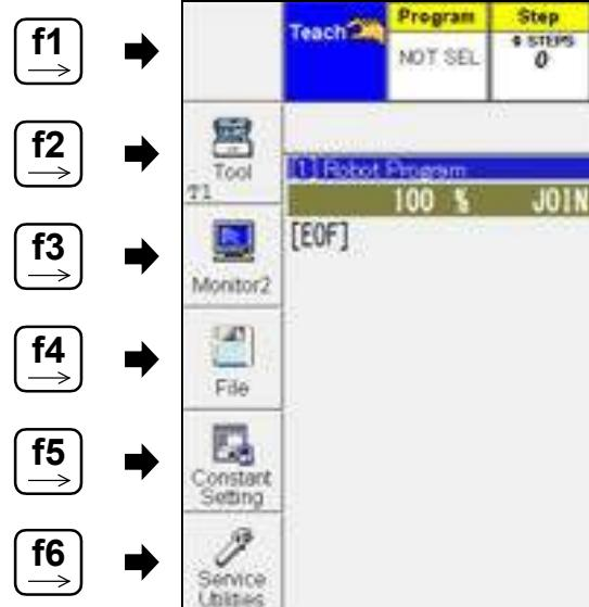
Normally, a function is selected by pressing one of the f1~f12 icons on its own. However, in some cases the key must be pressed together with [ENABLE].
