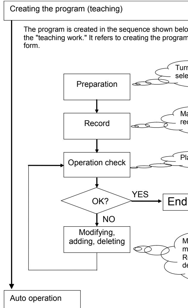
After the creation of the program has been completed, automatic operation is performed. When automatic operation is performed, the selected program is repeatedly played back.
