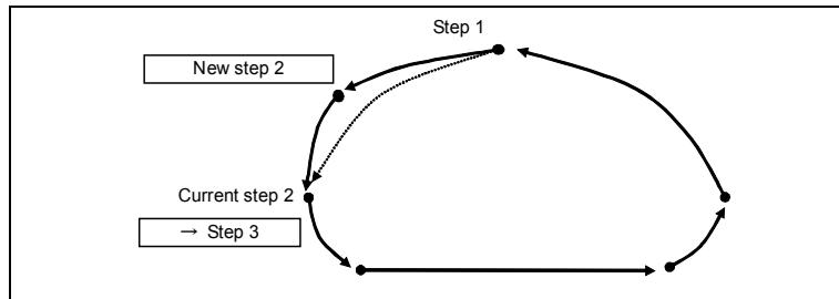
The position at which the command is added differs between <<Operating mode A>> and <<Operating mode S>>. The added position of the new step is "After the current step" for <<Operating mode A>>, and "Before the current step" for <<Operating mode S>>.
