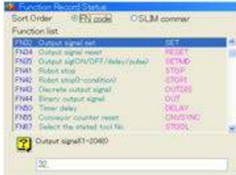
**2 Input the number of the output signal using the [Number input keys].**
