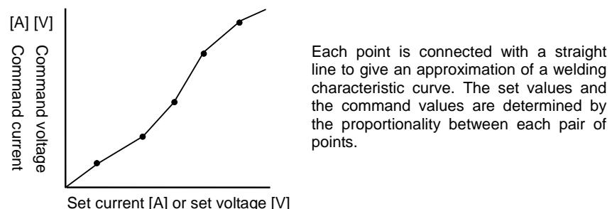
Fig. 2.5.1 Welding characteristic curve
