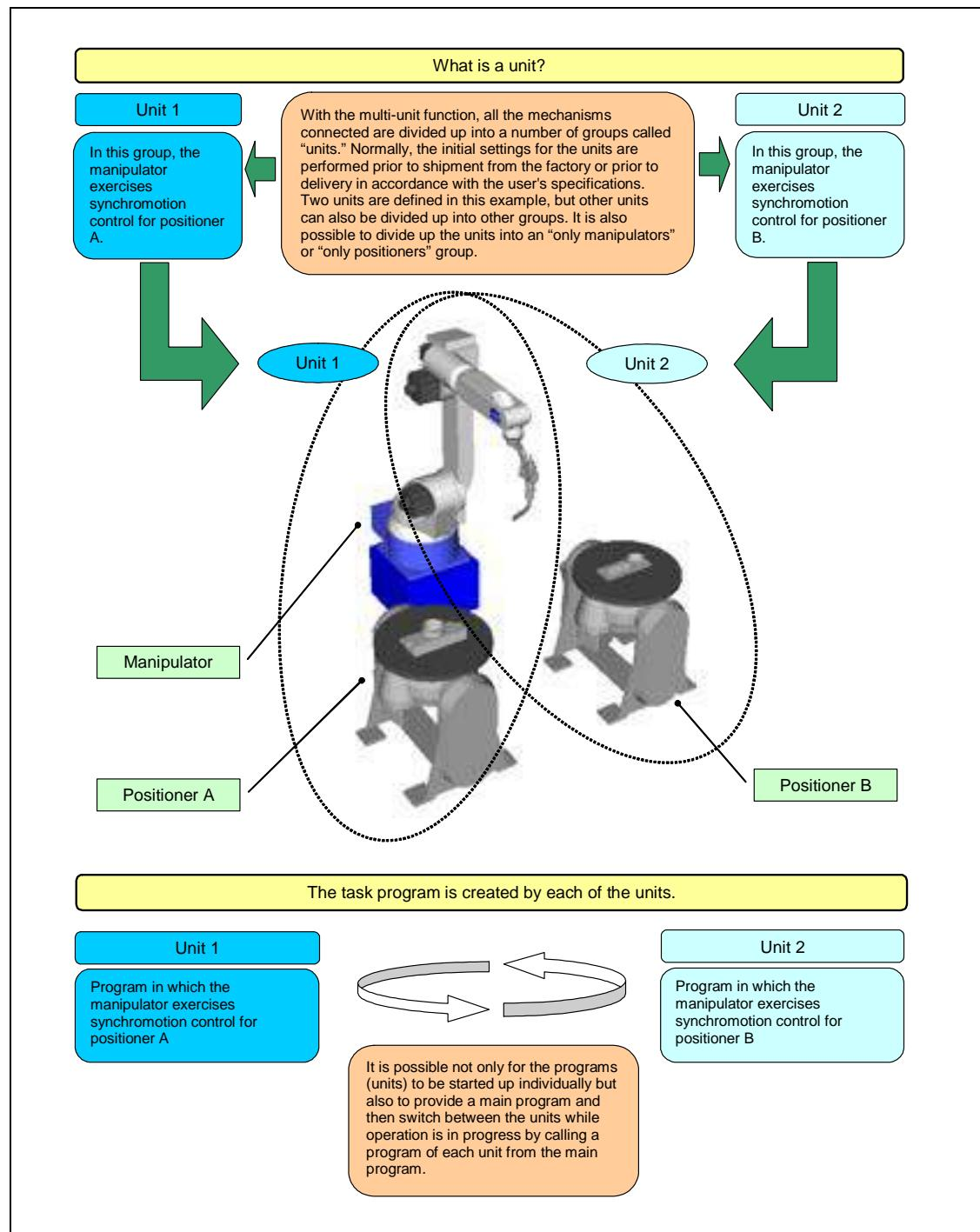
Fig. 1.3.2 Thinking behind the multi-unit (with multi-cooperation robots)
