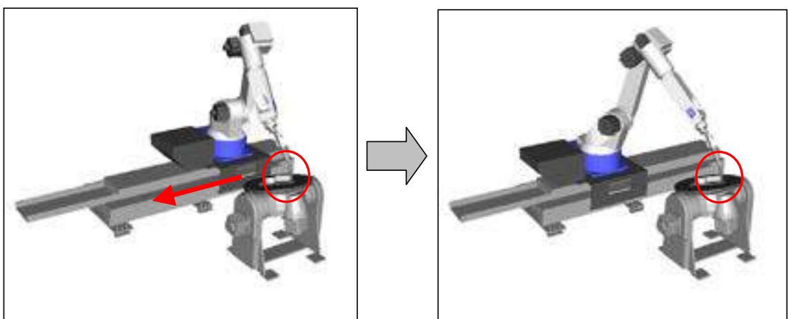
Fig 2.3.2 Cooperative manual operation when slider is moved
