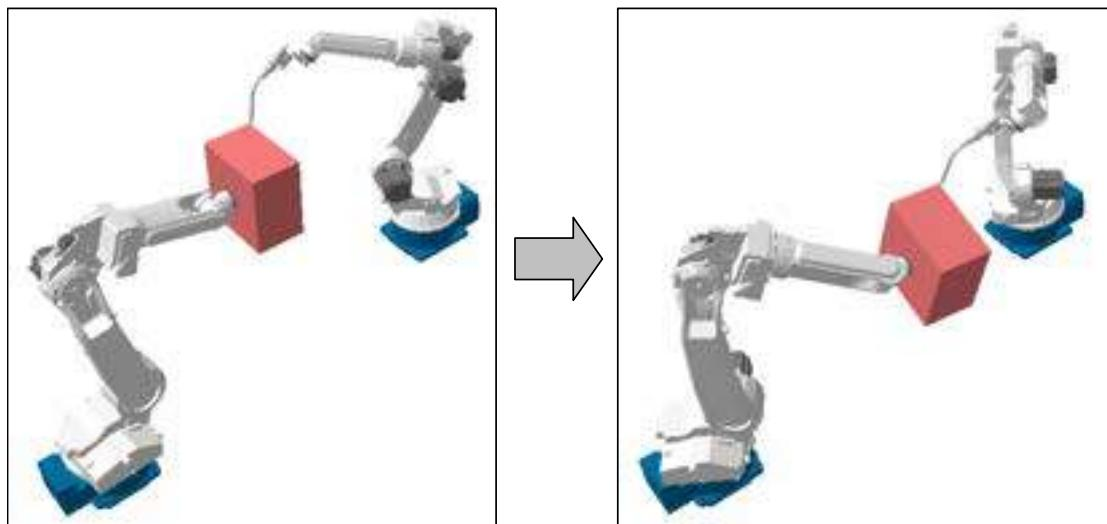
Fig 2.3.3 Cooperative manual operation by two manipulators
