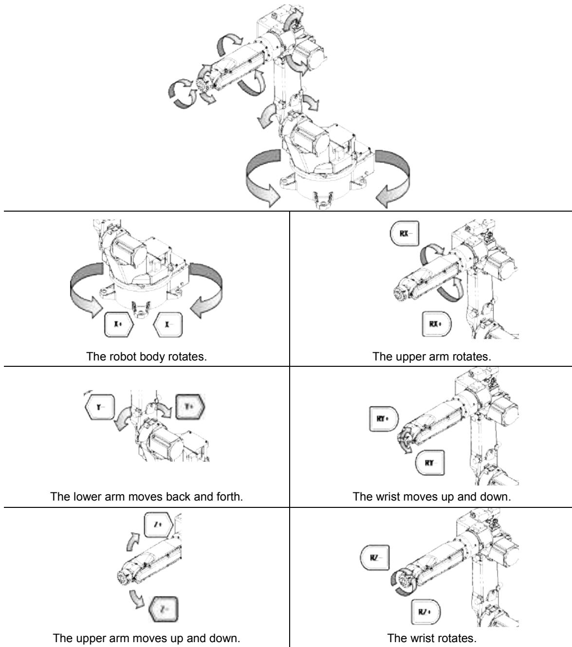
Fig. 3.4.1 Movement directions in the axis coordinate system
