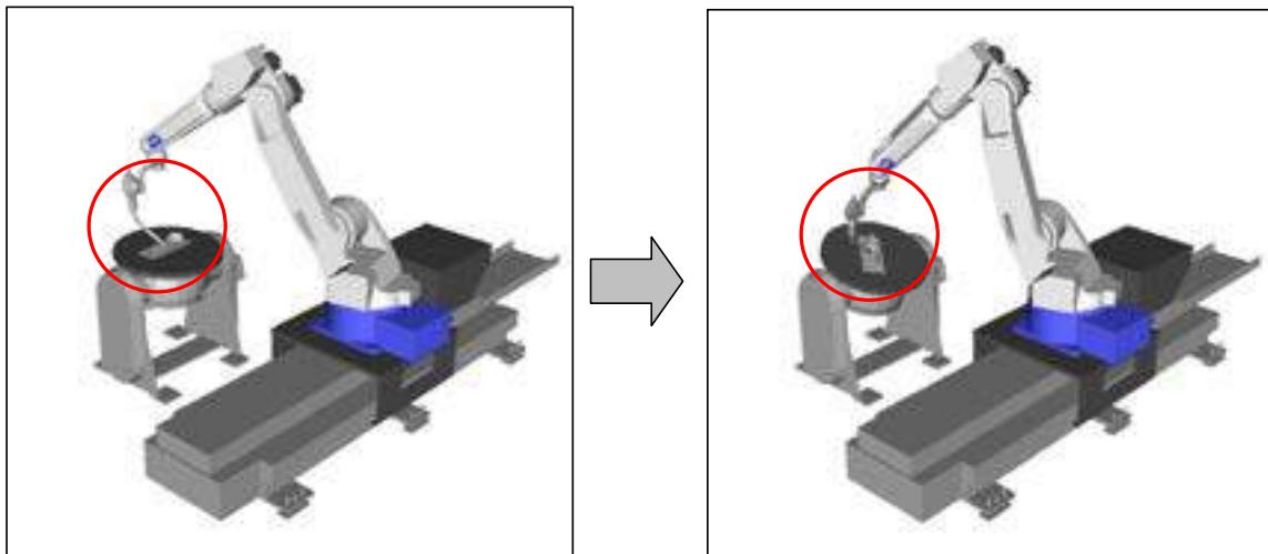
Fig 2.3.1 Cooperative manual operation when positioner is moved
