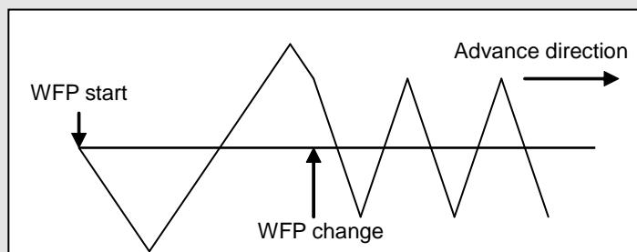
Fig. 3.4.1 Continuation of phase when conditions are changed
