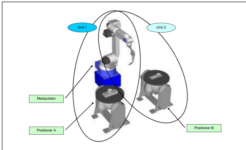
Fig. 1.2.4 Example of multi-cooperation robot configuration
