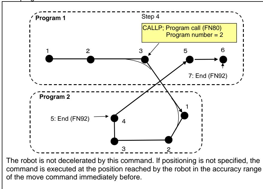
The program call can be executed again at the call destination (during program 2 in the above figure.) Up to 8 layers of calls can be executed. If calls exceeding 8 layers are executed, the "A2138 Wrong call command setting" alarm is detected during playback, and the robot stops.
