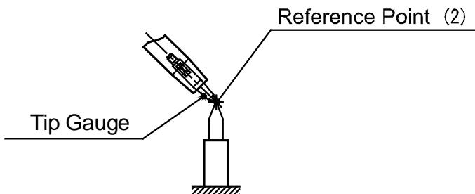
If there are issues such as deviation of the teaching point during playback, check the program and confirm the accuracy of the robot and torch.
