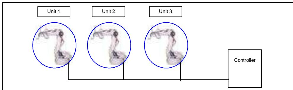
Fig. 1.2.1 Example of multi-unit configuration
