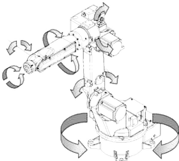
Fig. 1.4.2 Operating the axes separately (independent axis operation)
