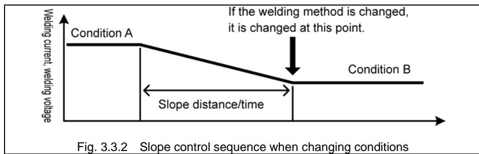
Fig. 3.3.2 Slope control sequence when changing conditions
