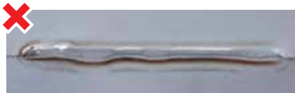
Insufficient heat input causes bead wandering
