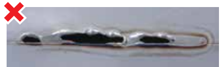
Excessive heat input cause burn through
