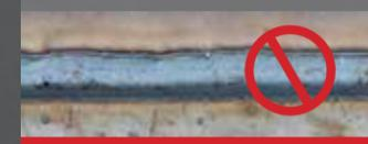
Conventional Pulse GMAW produces an erratic arc with excessive spatter and porosity.
