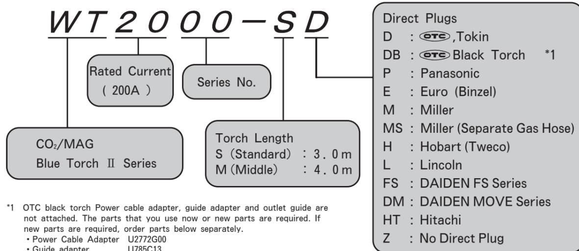
\*1 OTC black torch Power cable adapter, guide adapter and outlet guide are not attached. The parts that you use now or new parts are required. If new parts are required, order parts below separately.
